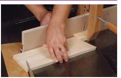
**Switch miter slots, not settings.** There's no need to change the blade angle when cutting opposite ends of a box side; just flip the board edge for edge and move the miter gauge to the other side of the blade. Label the inside and outside faces of each part and lay out all of the cuts to keep track of them. Also, use a stop block to index the second cut on each side.
