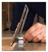
**Transfer that angle to the blade.** This is a good time to rip the top and bottom edges of the box sides, which usually are cut at this angle.
