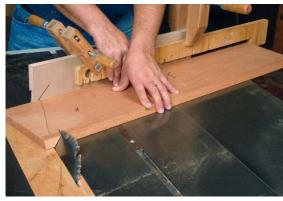
Again, lay out and label the sides to keep track of the cuts. Workpiece creep is especially a problem with these sharply angled cuts, so clamp on a stop block, or a stop stick.
