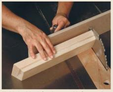
Hold the block in place and bring up the miter gauge. When the gauge is flush to the block, lock in the angle setting.
