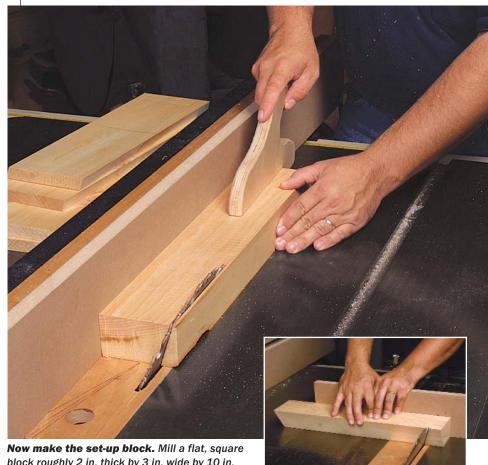
**Now make the set-up block.** Mill a flat, square block roughly 2 in. thick by 3 in. wide by 10 in. long. Then rip one edge (above) and crosscut the two ends at the slope angle (inset).
