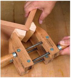
**Miter-joint clamping strategy.** Rip some scrap stock at the current blade angle and glue these blocks onto the workpieces. Use these clamping cauls to draw the joint tightly together. The blocks can be pared away later.
